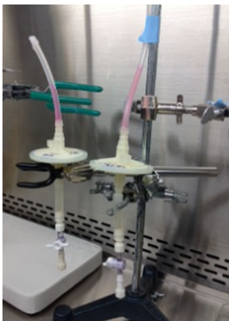
Fig. 3 Example of the capsule filter experiment set-up. Sterile tubing with sterile Luer lock fittings are attached to hold and isolate the S. marcescens culture from the environment during incubation. The pink coloration in the input medium results from S. marcescens growth
